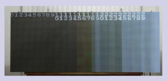
LED Wall Hardware: An indoor 6 mm pitch LED wall with a resolution of  $320 \times 180$  pixels, driven by Linsn's transmitter and recievers.
